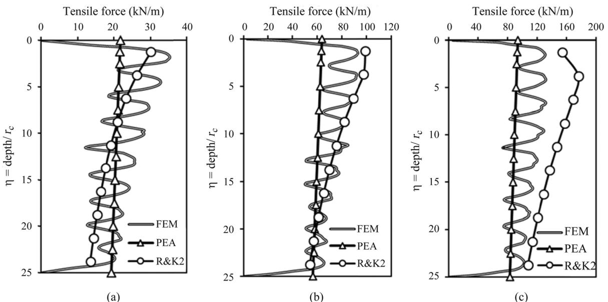
**Figure 2** - Tensile force vs. depth ratio for different geosynthetic stiffness: (a) Tensile force for  $J = 500$  kN/m, (b) Tensile force for  $J = 2000$  kN/m, (c) Tensile force for  $J = 4000$  kN/m.
