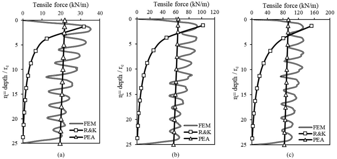
**Figure 1** - Tensile force vs. depth ratio for different geosynthetic stiffnesses; (a) Tensile force for  $J = 500$  kN/m, (b) Tensile force for  $J = 2000$  kN/m, (c) Tensile force for  $J = 4000$  kN/m (Fig. 5 after Alkhorshid *et al.*, 2018).
