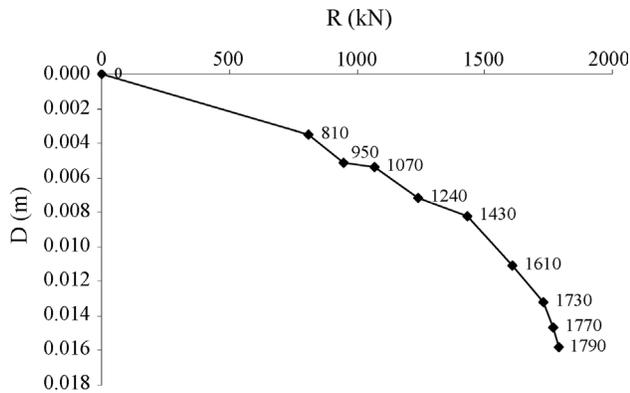
**Figure 3** -  $R$  vs.  $D$  graph of a driven pile (modified from Aoki, 2000).
