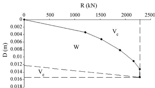
Figure 1 - The strain energies that form part of the mobilized static resistance ( $R$ ) vs. maximum displacement ( $D$ ) curve of DIET.
