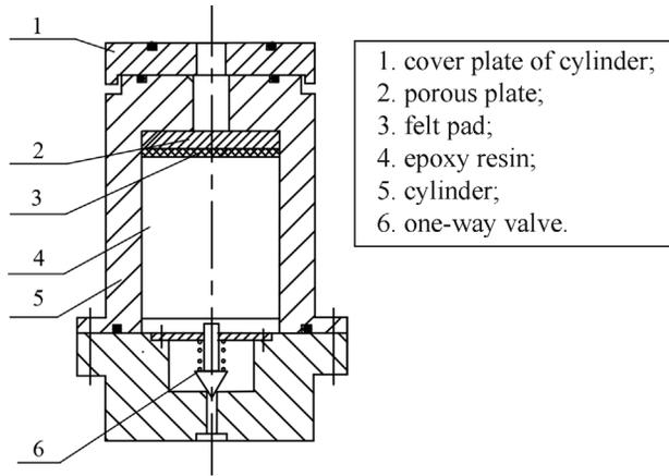
Figure 1 - Patented device in the experimental system.
