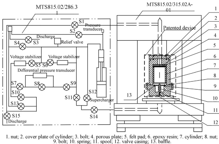
Figure 2 - Coupled assembly used in the experiment (MTS815.02 with a developed patented device).
