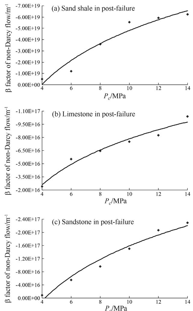
**Figure 4** - Relationship between the  $\beta$  factor of the non-Darcy flow and the confining pressure ( $P_c$ ) for the three rock types.
