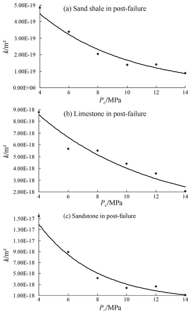
**Figure 3** - Relationship between the non-Darcy permeability ( $k$ ) and the confining pressure ( $P_c$ ) for the three rock types.
