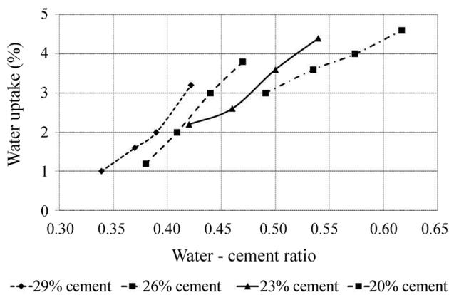
**Figure 1** - Capillary absorption study conducted by Schulze (1999).
