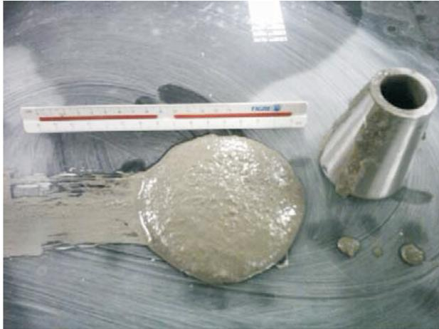
Figure 3 - Mini-slump test (Laister, 2012).
