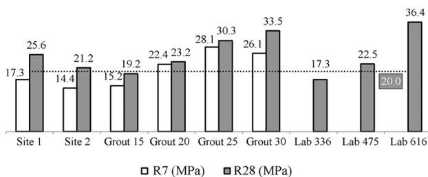
Figure 4 - Axial compressive strengths of the mortars studied (Laister, 2012).
