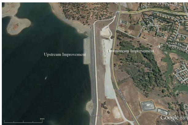
**Figure 7** - Aerial view of Mormon Island Auxiliary Dam as it appeared in August 2013. Critical section over potentially liquefiable foundation material extends about 300 m from the left abutment (Google Earth, Imagery Date 8/13/2013).
